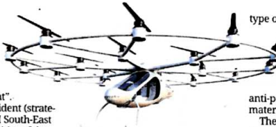
Volocopter's flagship two-seater drone is designed for use as an autonomous air taxi in large cities. — Reuters
